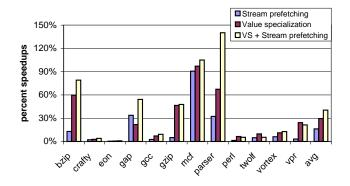
Fig. 6. Performance of value specialization with hardware prefetching
